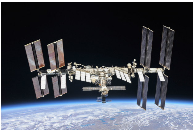
A complete view of the ISS as of October 4, 2018, taken from the Soyuz capsule of the departing crew of Expedition 56 from their Soyuz capsule. This structure was built by materials launched into orbit by 37 United States Space Shuttle missions and 5 Russian Proton and Soyuz rockets, and assembled and maintained by 230 spacewalks, with more to come! Credit: NASA/Roscosmos More info: bit.ly/issbasics and stargazing and satellite tracking apps.
